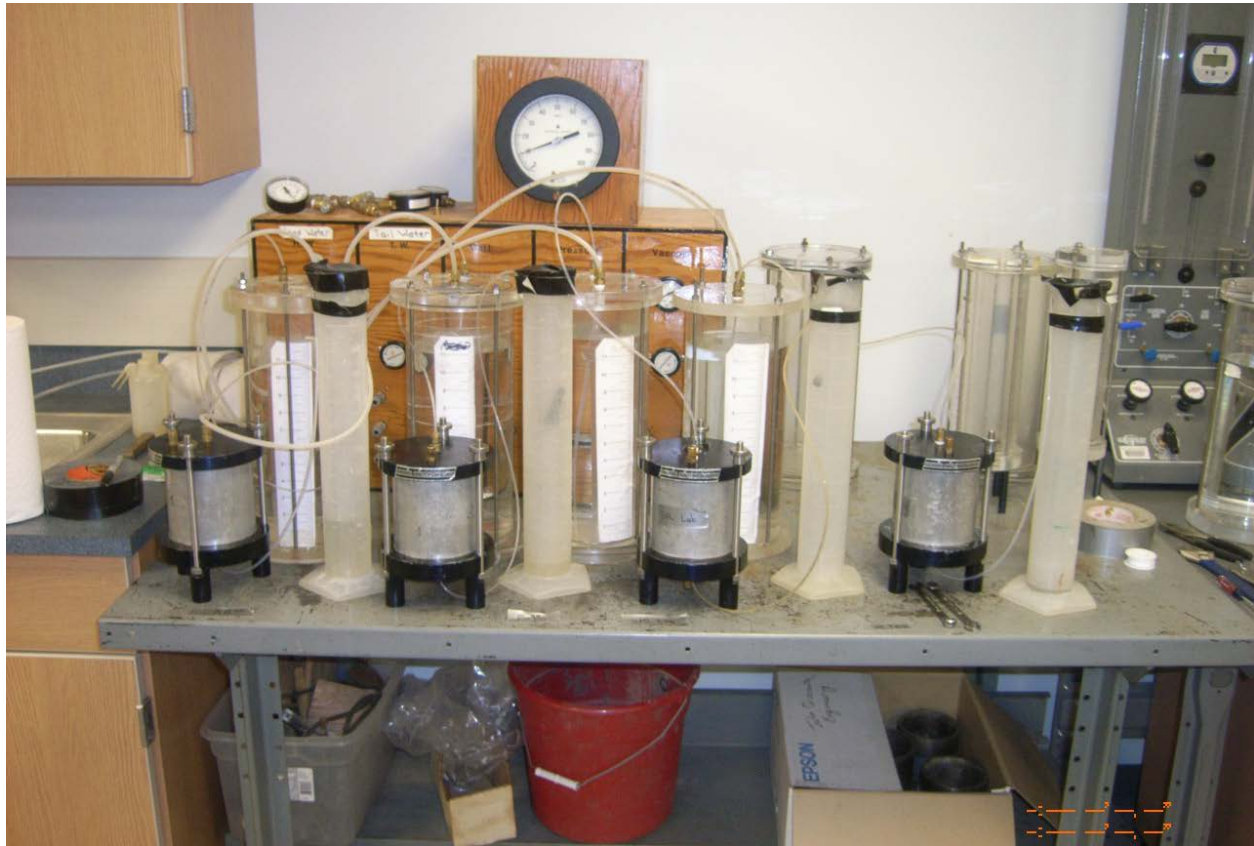
Figure 35: Hydraulic Conductivity Testing
