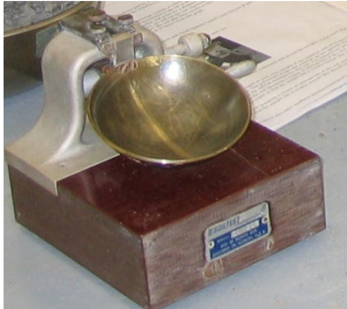
Figure 29: Liquid Limit Device (Casagrande Cup)
