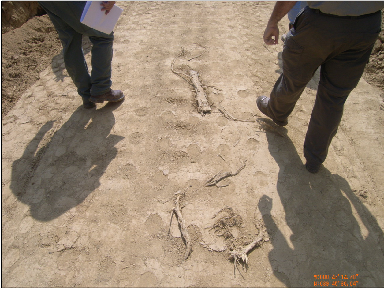
Figure 21: Woody Debris in Soil Lift
